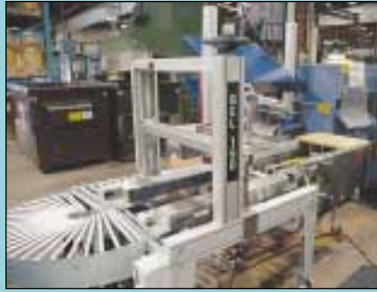
Belcor Automatic Carton Erecting & Box Taping Line
