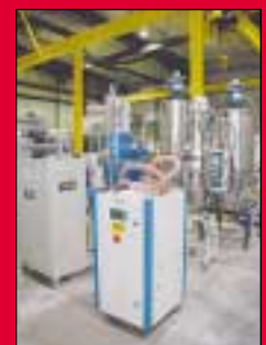
Partial View Dry Air and Comet Dehumidifying Dryer Systems
