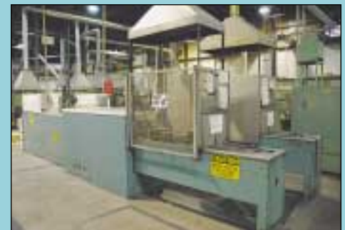
6" Wide CI Hayes Type LSC Continuous Mesh Belt Electric Fired Heat Treat Furnace
