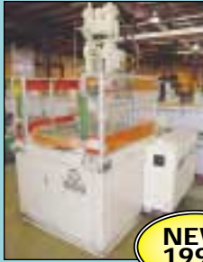
55 Ton Multiplas Model V3-6R-55T-33LDC Vertical Clamp Rotary Table Plastic Injection Molding Machine
