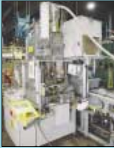
(2) 30 Ton X 2 Oz. Lawton Model 30T Vertical Gap "Book" Style Mold Injection Molding Machines
