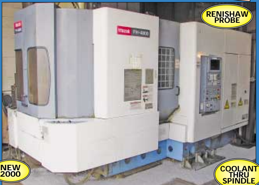
Mazak Model FH-4800 Four-Axis Two-Pallet CNC Horizontal Machining Center
